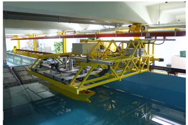
Fig 15 The high speed towing carriage after test setup
