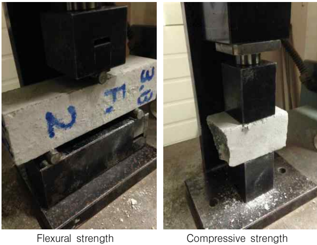
Figure 5. Flexural strength and compressive strength test
