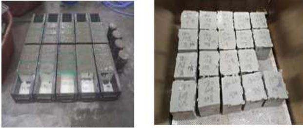
Figure 3. Manufacturing of specimens for direct shear test
