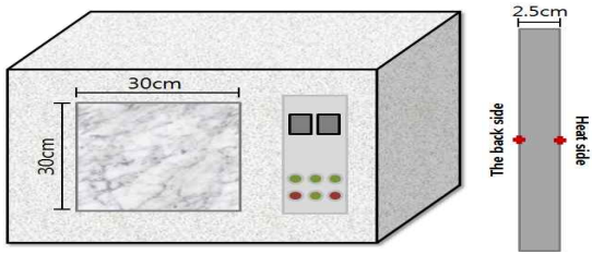
Figure 5. Heating experiment mimetic diagram and measure point
