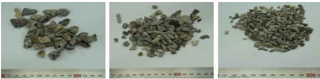
Figure 3. The image of the dry process bottom ash
