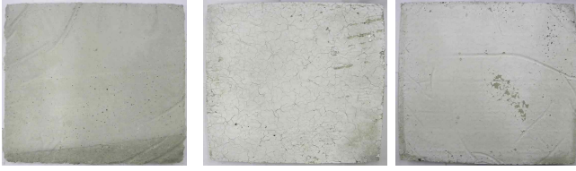
Figure 13. After (the first the left) former heating and heating surface condition
