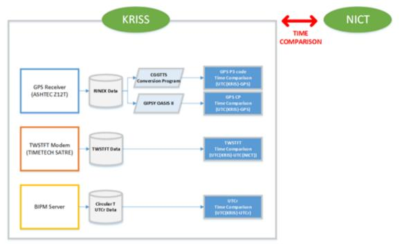
Fig. 3. Methods for time comparison.
