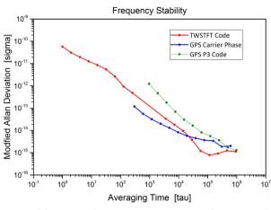
Fig. 8. Stabilities ( $\tau = 1$  s) between UTC(KRIS) - UTC(NICT) by TWSTFT code, GPS P3 code and GPS carrier phase.
