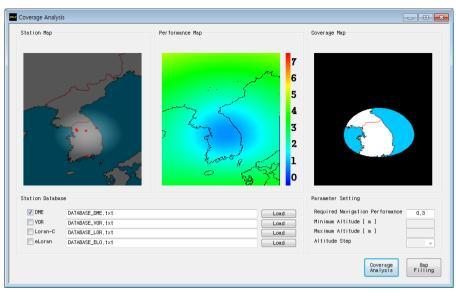
Fig. 11. Coverage analysis GUI.
