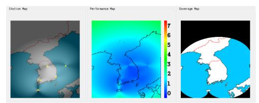
Fig. 19. Coverage analysis result of DME/eLoran.
