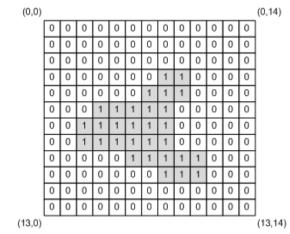
Fig. 9. Regions where a navigation signal sources can be located.
