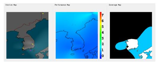
Fig. 16. Loran-C coverage analysis result.
