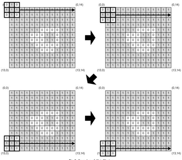
Fig. 5. Procedure of dilate filtering.
