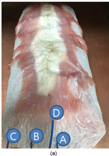
Figure 7. Frozen pork thawed by (a) parallel type and (b) curved electrodes with a chamber temperature of -20^{\circ}\text{C} .
