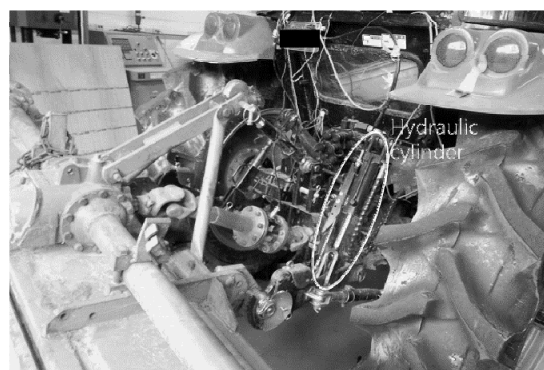
(b) Hydraulic cylinder as an actuator of horizontal control system
