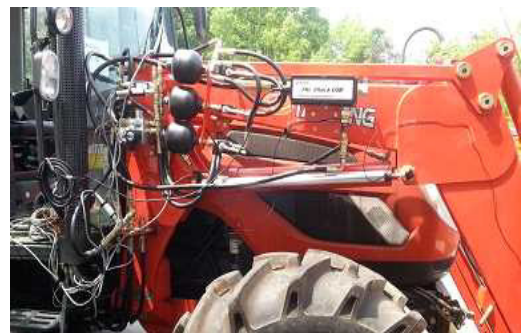
Fig. 12 View of components of the boom suspension mounted on the FEL
