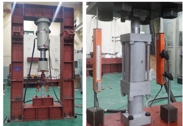
Fig. 5. Dynamic experimental configuration of proposed damper.
