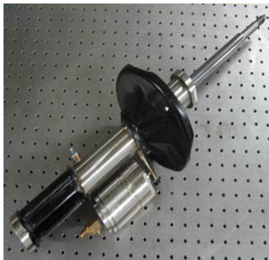
Fig. 2 Manufactured ER damper
