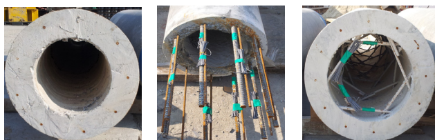
(a) PHC pile for connection type A (b) PHC pile for connection type B (c) Composite PHC pile
