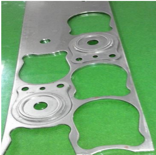
Fig. 12 Strip layout of a 2 cavity seat recliner
