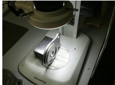
Fig. 14 Sheared surface measurement of the seat recliner product
