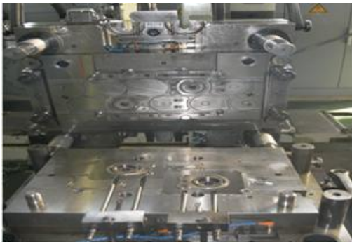
Fig. 10 Die assembly of a seat recliner
