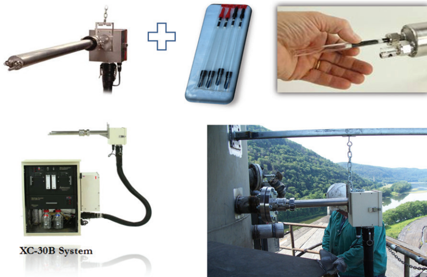
Fig. 5. Sorbent trap measurement system.
