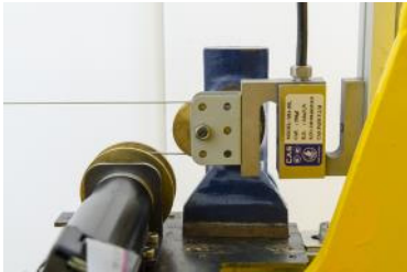
(c) actuator system for tension control with loadcell
