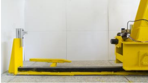
(a) photo of overall tension control system
