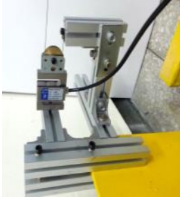
(b) loadcell installed on the opposite end side
