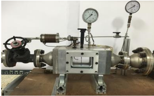
Fig. 2 Photo of the combustion chamber
