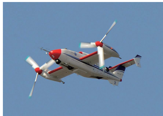
Fig. 1. Flight test in airplane mode of the Smart UAV [2]
