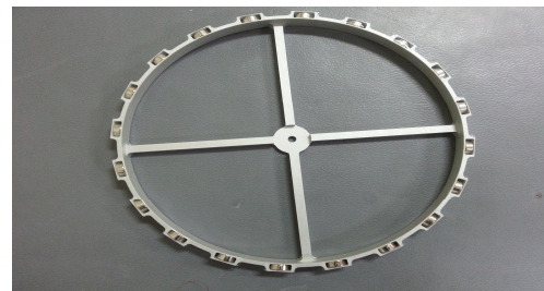
Fig. 8. Frame with magnets as many as the number of poles in the ring
