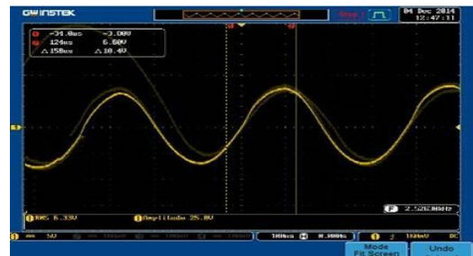
Fig. 7. Experimental results of electric generation with the consideration of phase difference (three-phase) in induced current
