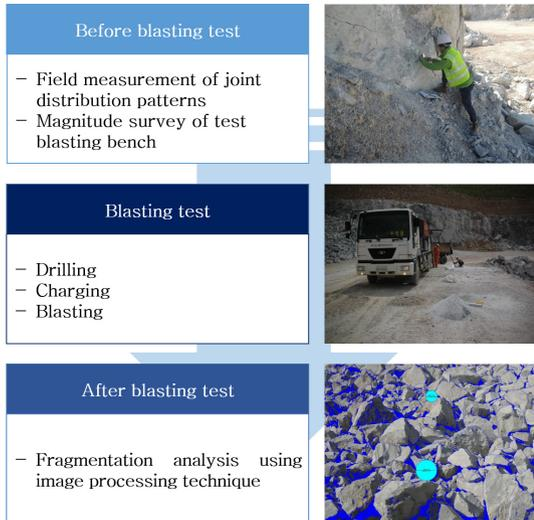
Fig. 2. Process of field survey and blasting test
