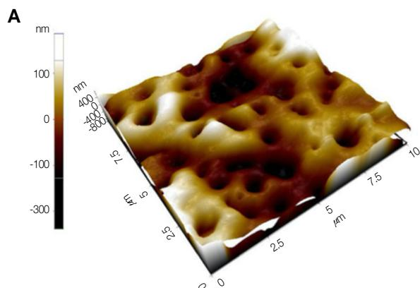
**Fig. 2.** The results of surface roughness measured by AFM ( $10 \mu\text{m} \times 10 \mu\text{m}$ ). (A) Anodized titanium disc, (B) Anodized titanium disc coated with 40  $\mu\text{l}$ rhTGF- $\beta$ 2 (500 ng/ml per disc).
