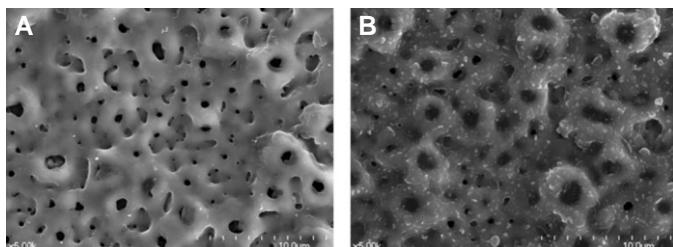
**Fig. 1.** SEM image of anodized titanium implant coated by electrospray ( $\times 5,000$ ). (A) Anodized Ti disc, (B) Anodized Ti disc coated with 40  $\mu\text{l}$ rhTGF- $\beta$ 2 (500 ng/ml) sub-micron particles by electrospray technique.
