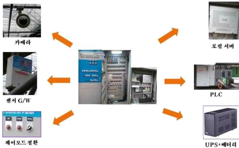
Fig. 5 Views of the greenhouse monitoring and control system.
