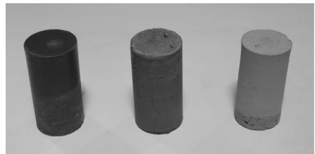
Fig. 13. Specimens cured for 170 days (soaking, wetting, drying)
