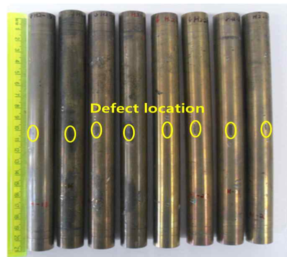
Fig. 1. Defect tubes for ECT signals analysis.
