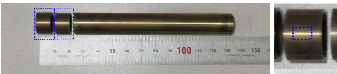
Fig. 3. The specimen for oxide analysis of the surface.
