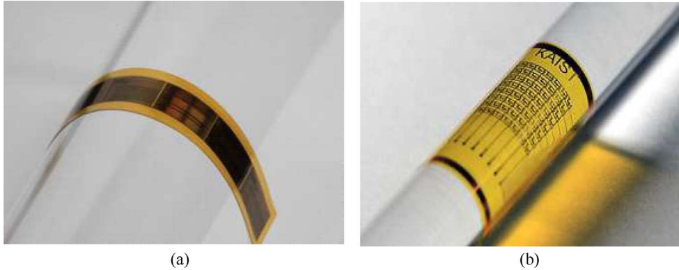
Fig. 4. Pictures of flexible memory developed by (a) Hanamicon Co. in Korea. (b) KAIST
