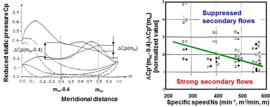
Fig. 6 Guide line to achieve suppressed meridional secondary flows
