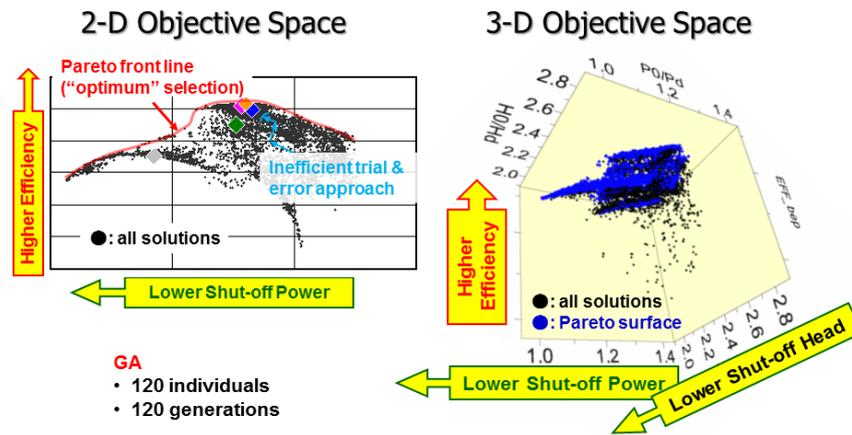
Fig. 8 Visualization of Pareto front on 2-D and 3-D objective space
