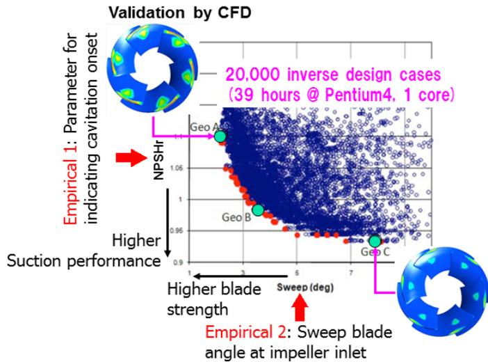
Fig. 10 Multi-objective optimization based on empirical objectives
