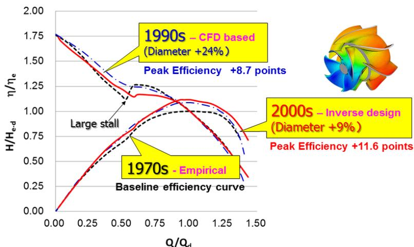
Fig. 3 Performance improvements of a mixed-flow pump stage during the last 30 years
