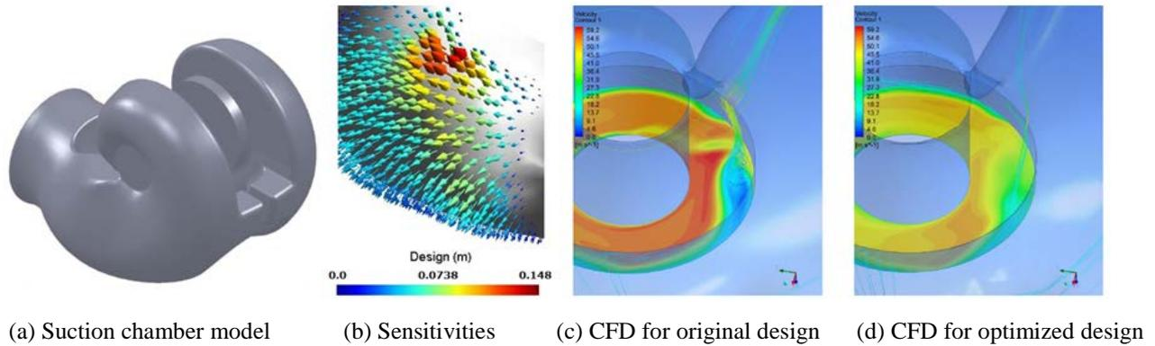
**Fig. 12** Optimization of a double suction chamber for a centrifugal pump
