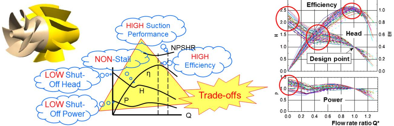
Fig. 7 Definition of multi-objective optimization
