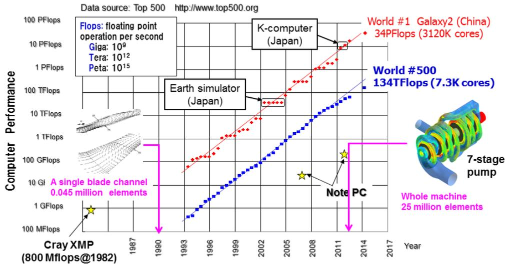
Fig. 1 Advancements in computer performance and CFD models
