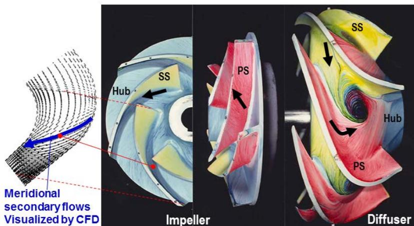
Fig. 4 Secondary flows visualized by multi-color oil-film method (conventional design pump)
