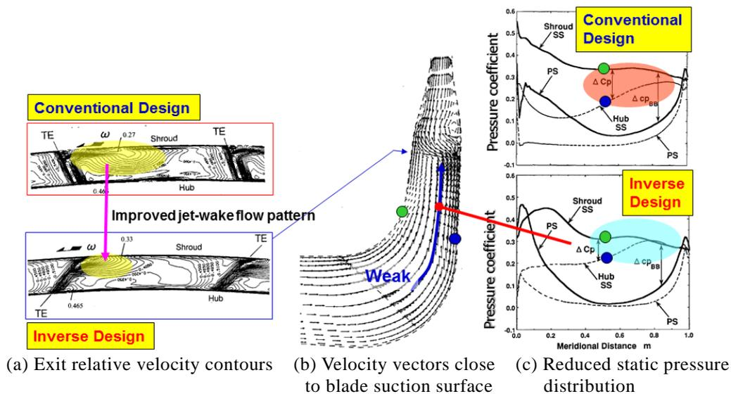
**Fig. 5** Impeller secondary flow control by 3-D inverse design method
