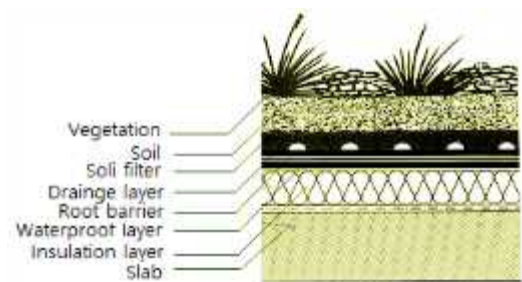
Figure 1. Composition of typical green roof system
