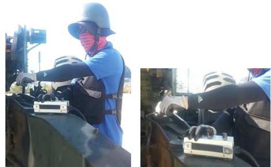
Figure 8. Motor-Driven Manipulation of Firing Elevation Wheel
