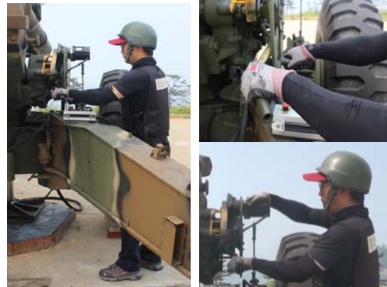
Figure 7. Manual Manipulation of Firing Elevation Wheel
