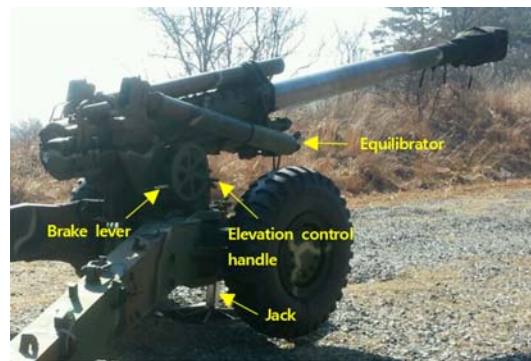
Figure 3. 155mm Towed Howitzer
