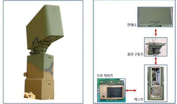
Fig. 2. Figuration of surveillance radar
