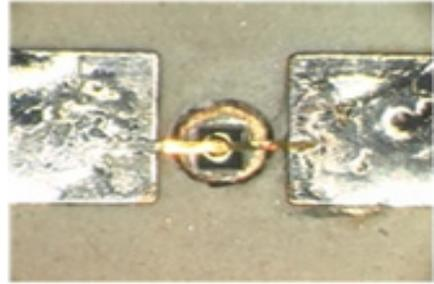
Fig. 6. PIN diode applied to Limit&STC Assembly
