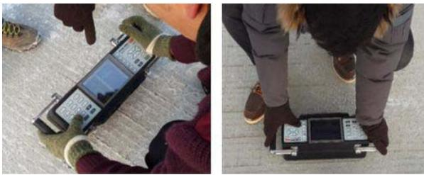
Fig. 9 Inspection of Rebar with MIRA and Rc-Radar
