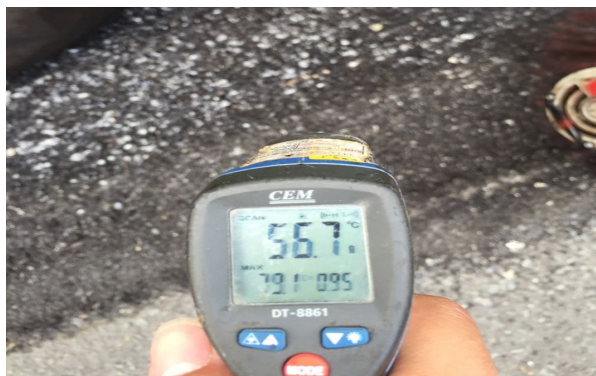
(b) Measured Temperature After Milling
