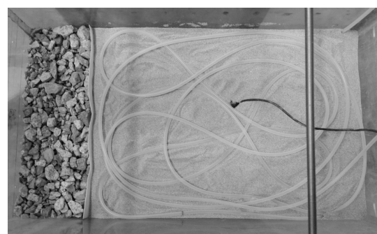
(b) Setting of heating wire and 5TE sensors
