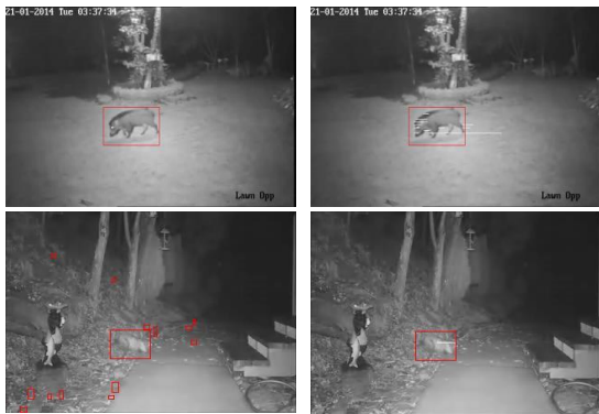
Fig. 4. Remove noise. The left column is the foreground detection. The right column is the foreground detection using Optical flow.
