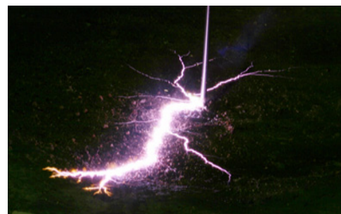
Fig. 1. Photograph of surface flashover from the driven ground rod impressed by a lightning impulse voltage.
