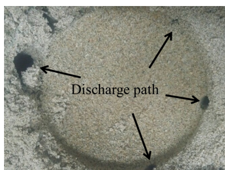
Fig. 10. Photograph of soil discharge impacts
