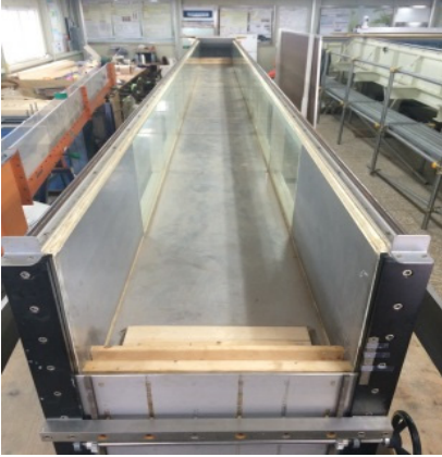
Fig. 2. Photograph showing a flume for laboratory experiments in this study.
