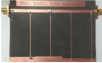
Fig. 7. Photograph of fabricated negative group delay circuit.
