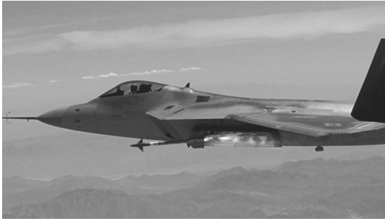
Fig. 1. An AIM-9 missile is launched from a internal weapon bay of a F-22 stealth fighter
