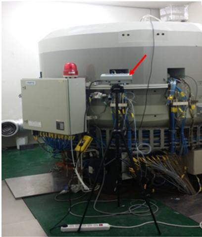
Fig. 5 Gamma dose rate from the target was measured with an area monitor device marked by a red arrow
