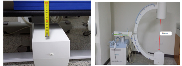
(c) Distance to the Tube and Procedures Table (d) Distance to the Tube and Detector
