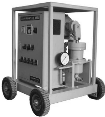
Fig. 3. Vibration generator of CGVM system (Korean Geo-Environmental Society, 2013).
