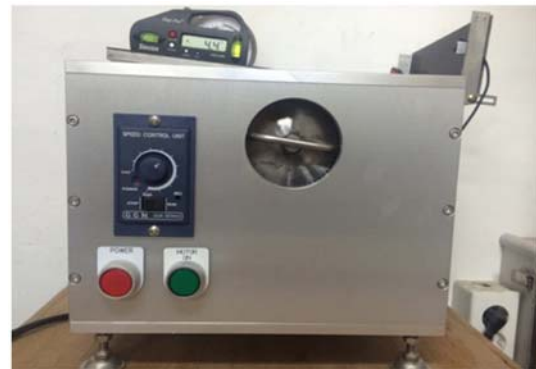
Fig. 9. Photograph of the tilt test machine used in the present study.
