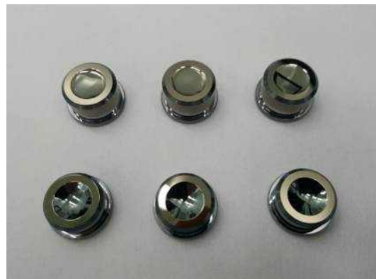
Fig. 9. 2 nd lens(up) and mold core
