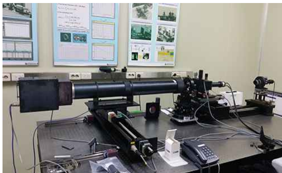
Fig. 10. Tester of MTF at KRISS
