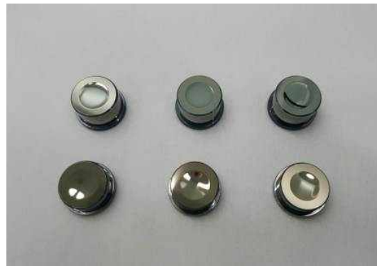
Fig. 8. 1 st lens(up) and mold core
