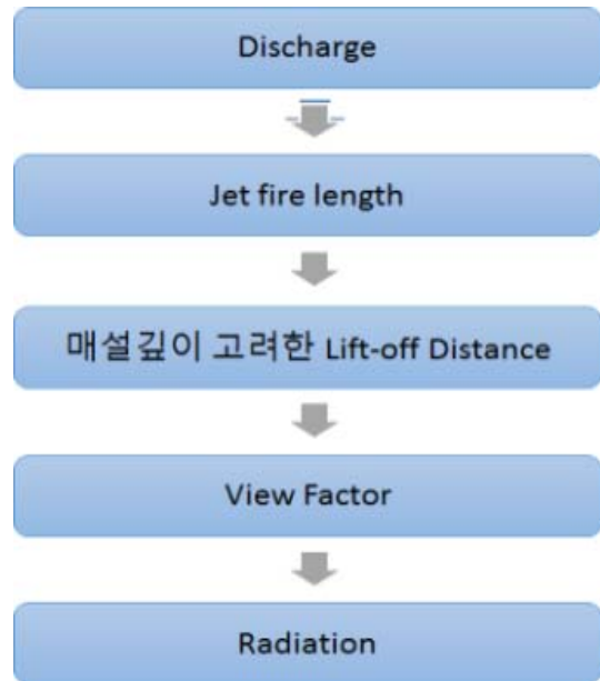
Fig. 3. Procedure of buried pipeline jet fire model.
