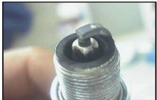
Fig. 3. Pollution condition of spark plug.
