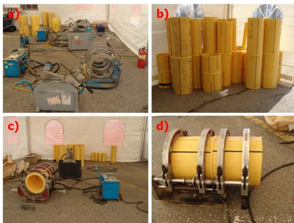
a) butt fusion machine b) after butt fusion c) butt fusion system d) setting into the clamp
