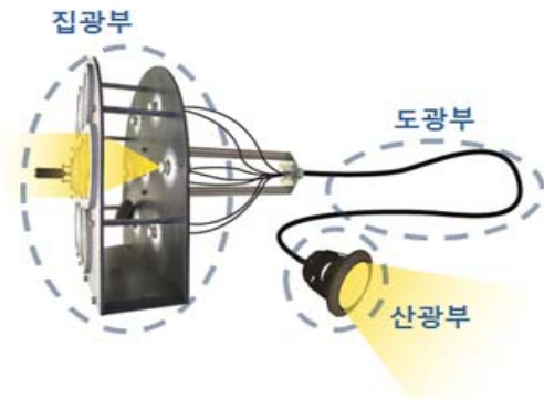
Fig. 6. Structure of the WDF[26]
