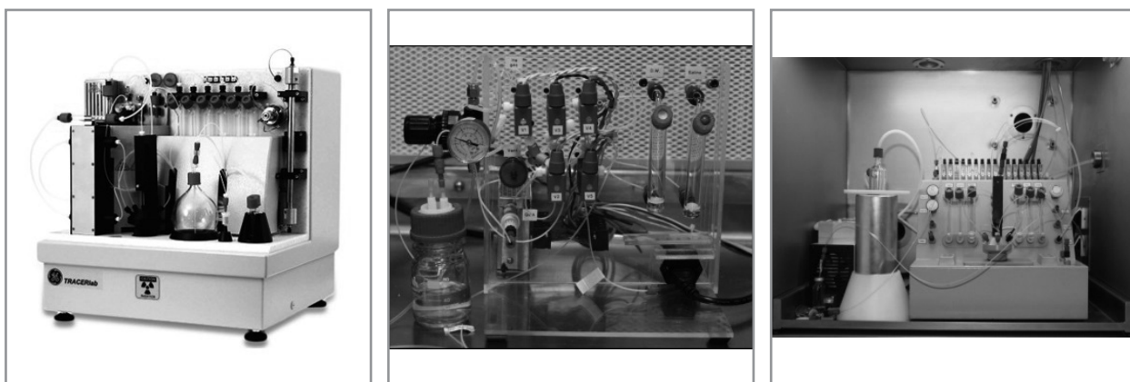
Figure 1. Synthetic modules: TRACERlab FXC-pro (left), hand-made NaF module (middle) and FDG auto-synthesizer (right)
