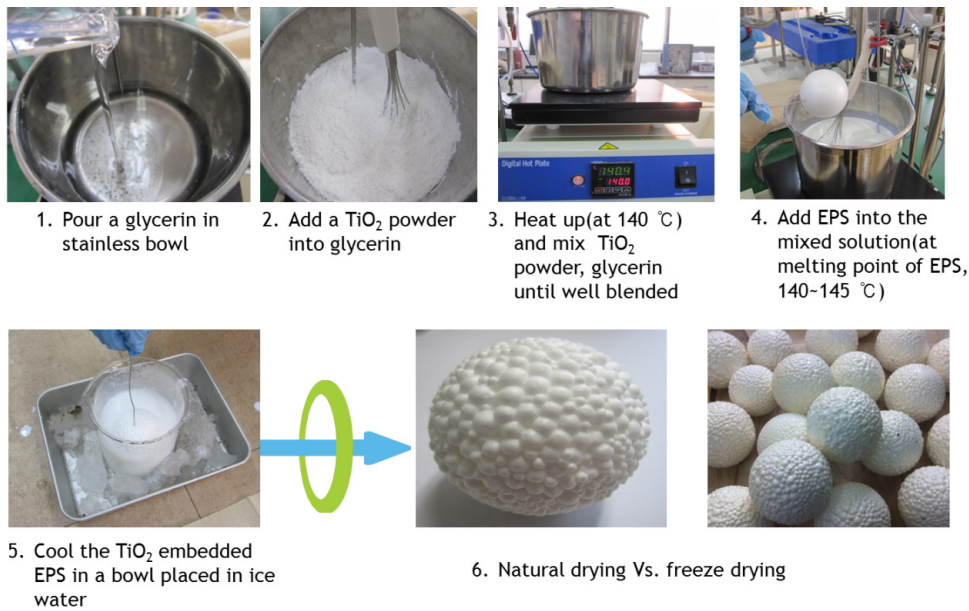
Fig. 1. Production procedures of \text{TiO}_2 -immobilized EPS balls used in this study.
