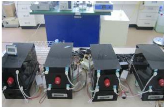
Fig. 2. Pictorial view of the batch photocatalytic reactor (from right to left: 1. UV only, 2. intact EPS balls with UV, 3. \text{TiO}_2 -immobilized EPS balls with UV, 4. Only \text{TiO}_2 -immobilized EPS balls without UV).
