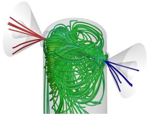
Figure 3. Streamline of resin and hardener flow inside the mixing chamber (The red, blue and green color signifies the resin, hardener and mixture of them, respectively).
