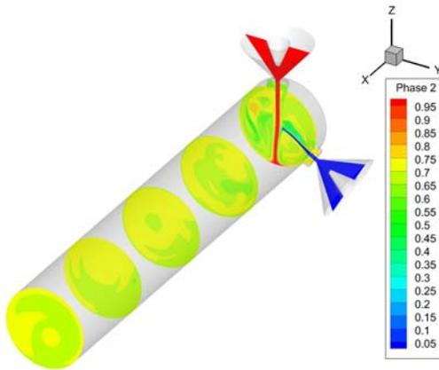
**Figure 6.** Contours of void fraction for resin phase (Phase 2) in different position in mixing head; Mixing ratio and nozzle diameter are 100:35 and 0.45mm, respectively.
