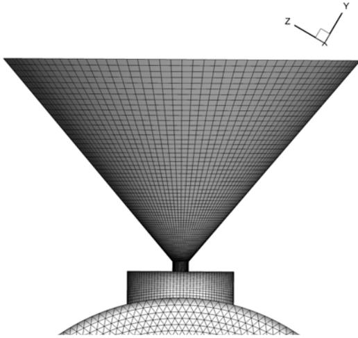
Figure 2. Nozzle geometry and structure mesh.
