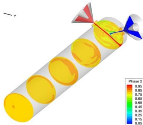
Figure 5. Contours of void fraction for resin phase (Phase 2) in different positions in mixing head; Mixing ratio and nozzle diameter are 100:35 and 0.3mm, respectively.
