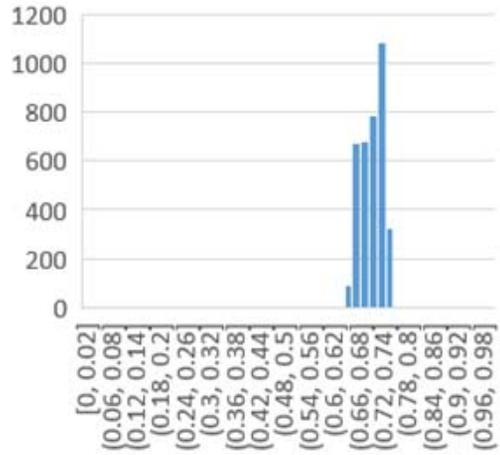
**Figure 9.** Histogram of void fraciton for resing ar the outlet of mixing head; the mixing ratio and nozzle diameter are 100:35 and 0.3mm, respectively.
