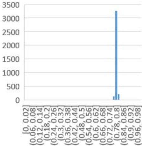
**Figure 8.** Histogram of void fraciton for resing ar the outlet of mixing head; the mixing ratio and nozzle diameter are 100:35 and 0.3mm, respectively.
