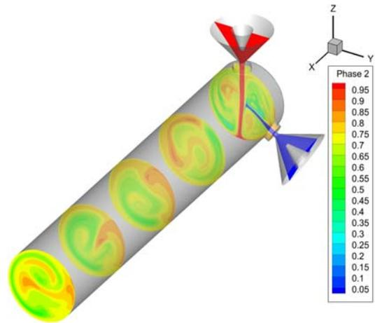
**Figure 7.** Contours of void fraction for resin phase (Phase 2) in different position in mixing head; Mixing ratio and nozzle diameter are 100:35 and 0.6mm, respectively.
