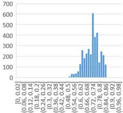
**Figure 10.** Histogram of void fraciton for resing ar the outlet of mixing head; the mixing ratio and nozzle diameter are 100:35 and 0.3mm, respectively.
