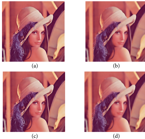
Fig. 1. Different effects of bilateral filter with fixed parameters: (a) \sigma_d = 5 , \sigma_r = 0.1 , (b) \sigma_d = 5 , \sigma_r = 0.3 , (c) \sigma_d = 20 , \sigma_r = 0.1 , and (d) \sigma_d = 20 , \sigma_r = 0.3 .
