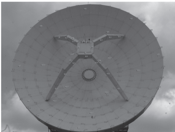
Fig. 2. Feature point labeling for control point surveying and acquisition of image coordinates (Kim et al. , 2015)
